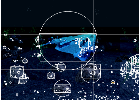
Figure 2: OpenCV methodology to draw bounding rectangles and circles around detected contours in an image.
