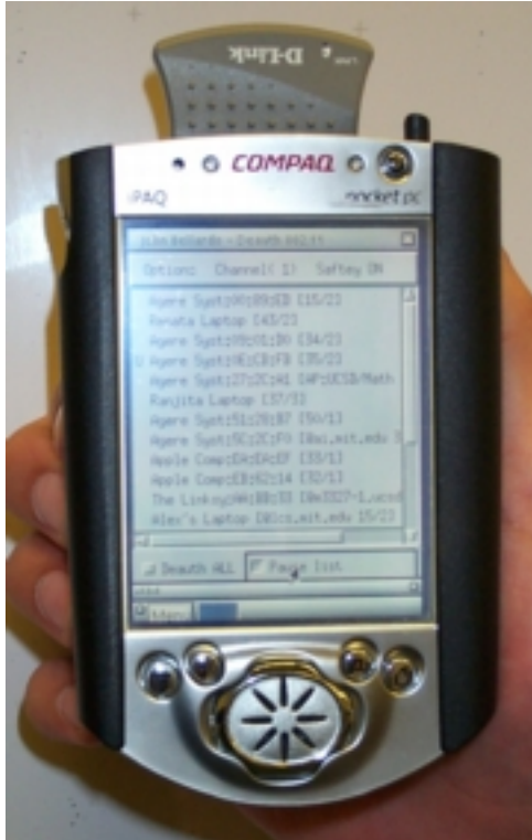
Figure 4: iPAQ H3600 with Dlink DWL-650 card, running Swat attack testing tool. Individual clients and AP's are identified either using MAC address or by passively monitoring the channel and extracting destination IP addresses and DNS names.
