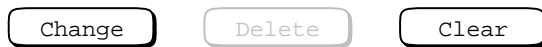
Figure 144: State of command buttons after user edits one or more data fields.
