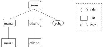
Target main has three dependencies. Two correspond to both rules and files. The third corresponds only to a rule. Each of the rules is recursively applied. The first, main.o, depends only on a file (namely, main.c). If the timestamp for main.c is newer than that of main.o (or if main.o does not exist), then the actions for main.o are executed. Otherwise, nothing happens. The rule for other.o works similarly. The rule for echo contains no dependencies, so its actions will be executed.
