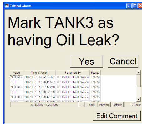
Figure 6: Detail screen for a critical alarm, in this case indicating that the pumper has seen oil on the ground. From here, the history for these actions can be seen ("SET" meaning that there's an oil leak, "NOT SET" meaning that the oil leak has been resolved), as well as being able to add any notes about the details of the oil leak to help cleanup crews.
