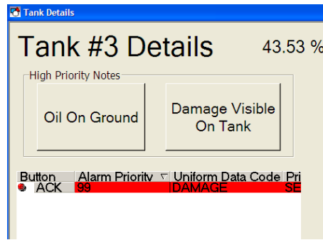
Figure 5: This tank has been previously marked as having damage. This can be an indicator for the pumper to more thoroughly inspect the tank for any oil leaks beyond what he would normally do.
