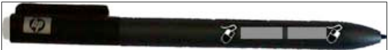
Figure 5: The modified stylus design with added mouse buttons and edited eraser color.
