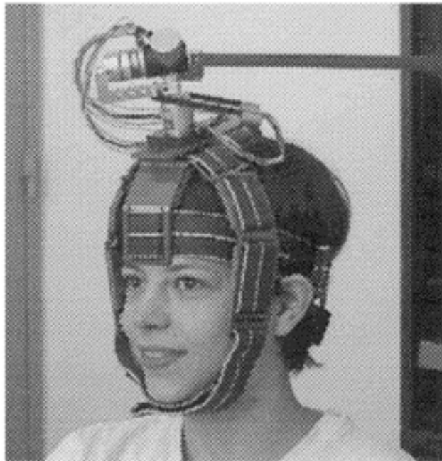
Figure 7. A complicated apparatus for tracking the movements and location of a user's head [40].
