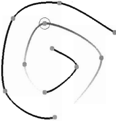
Figure 5.4: A single control point in a series of Catmull-Rom curves only locally affects the curve segments between its two succeeding and preceding control points in our implementation. Here, the influence of moving the selected control point is depicted with the strongest influence corresponding to red shading, and the weakest influence indicated by yellow shading.
