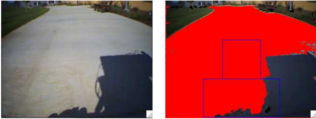
Figure 3. In this image, the algorithm incorrectly ignores the shadowed area. The number of shadow pixels in the background exceeds the number of pixels in the training area. This leads to incorrect classification.
