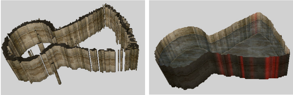
Figure 6: On the left is the geometric model of the House Dar T'ana (private home on Gozo) cistern before hole filling and on the right is the complete geometric model including uncertainty visualization of surfaces created via hole filling.
