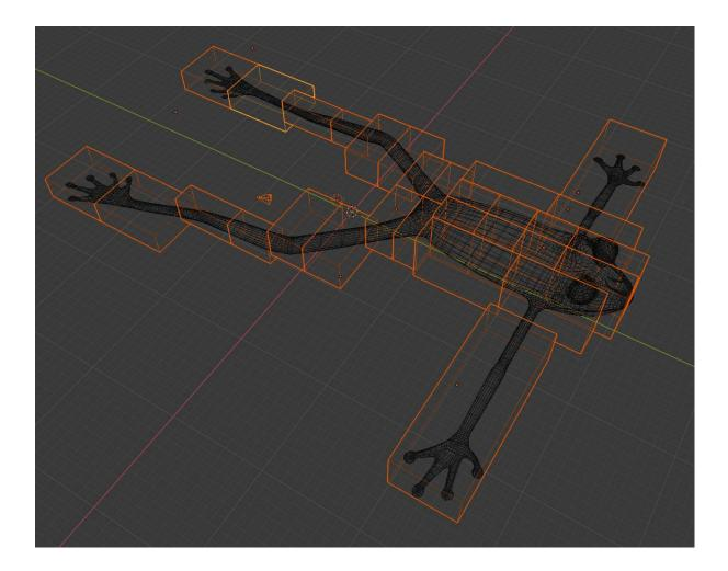
The preceding sequence represents 5 iterations of finding the bounding box, finding the center of mass, then dividing the box through a plane perpendicular to the long axis and recursing. If you imagine a point stored at the center of every pair of split boxes, upon connecting those points you should have a workable skeleton.
