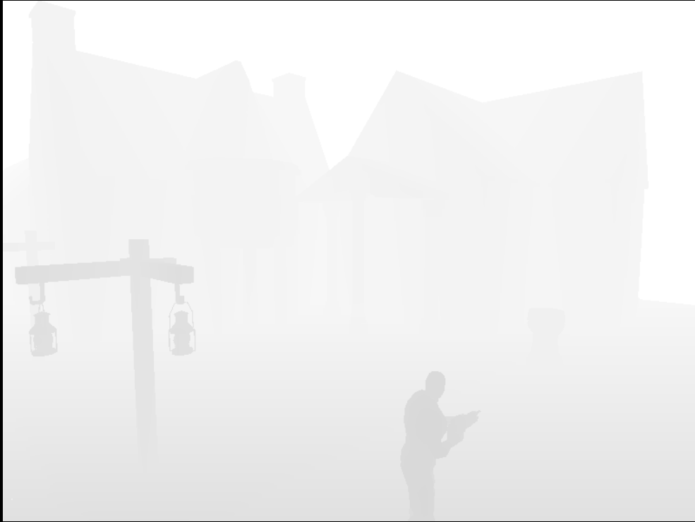
FIGURE 4—DEFERRED RENDERING DEPTH BUFFER (NON-LINEARIZED)
