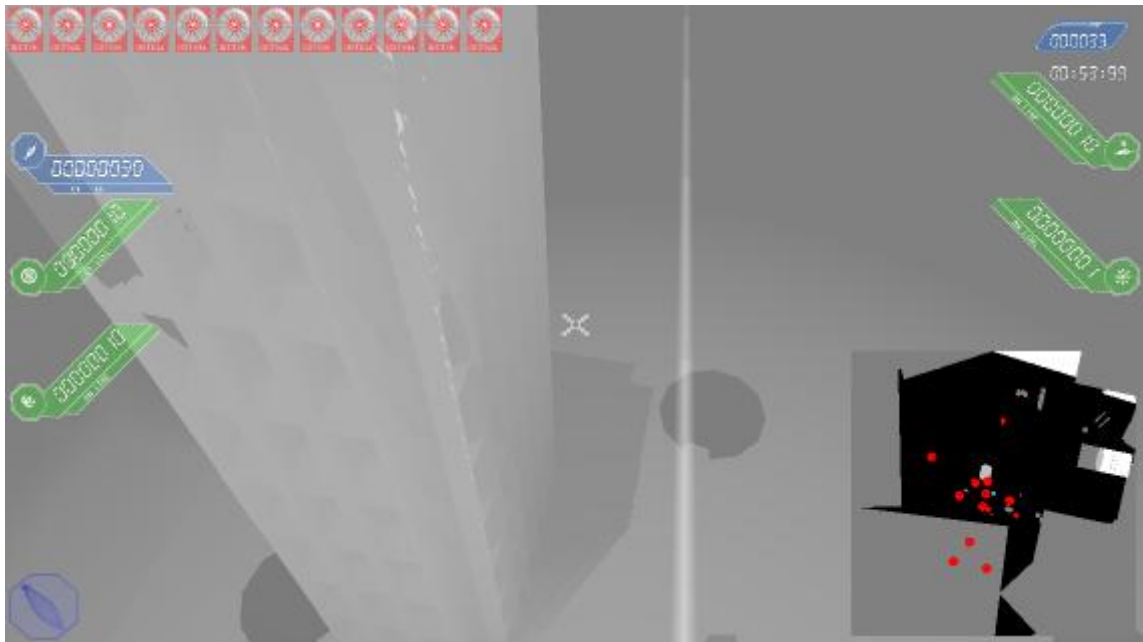
Figure 10: Light Depth read from shadow map. Darker is closer to the light.
